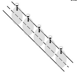
The typical deployment scenario for a road is 45-degree detection angle relative to the road.
